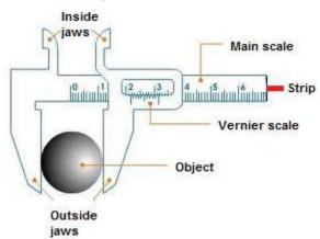
The main parts of vernier callipers and their functions are given below.
