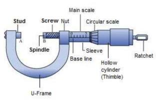
• The main parts of a screw gauge and their functions are given below.
